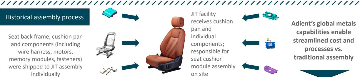
JIT facility receives cushion pan and individual components; responsible for seat cushion module assembly on site
